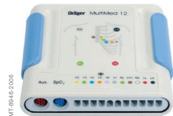
Infinity MultiMed 12 Pod Continuously monitors 12 leads of ECG and generates diagnostic reports.
